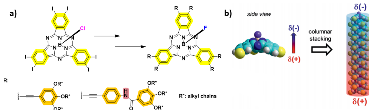
Figure 1. a) Chemical structure of the R 6 -SubPcs-F and b) molecular model of SubPc-based columnar stacks.
